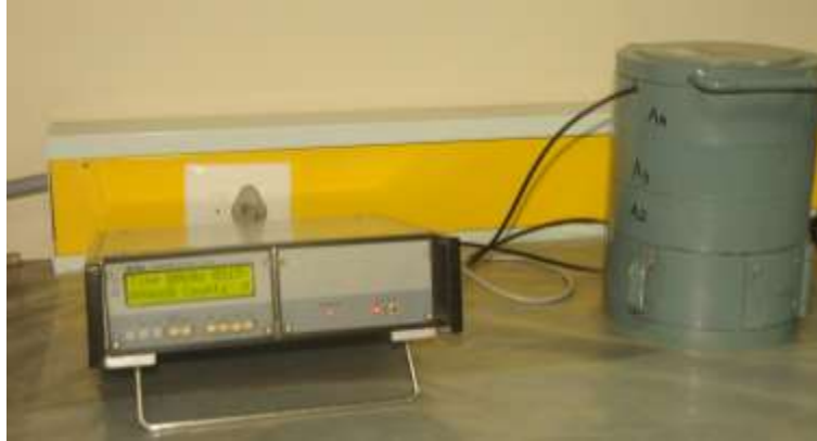
Figure 1. Working arrangement of a typical Beta counting system.
